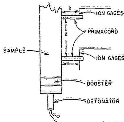
FIG. 1 DETONATION VELOCITY APPARATUS.
