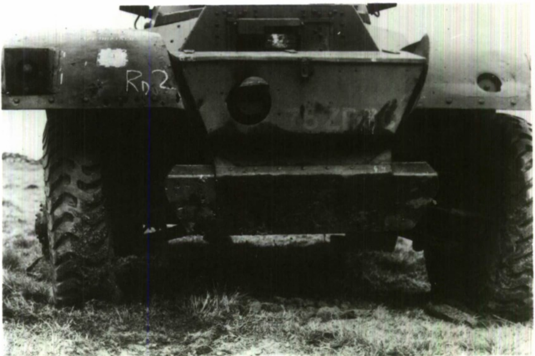
FIG. 2 NEAR MISS CLOSE TO THE FRONT OF THE VEHICLE
