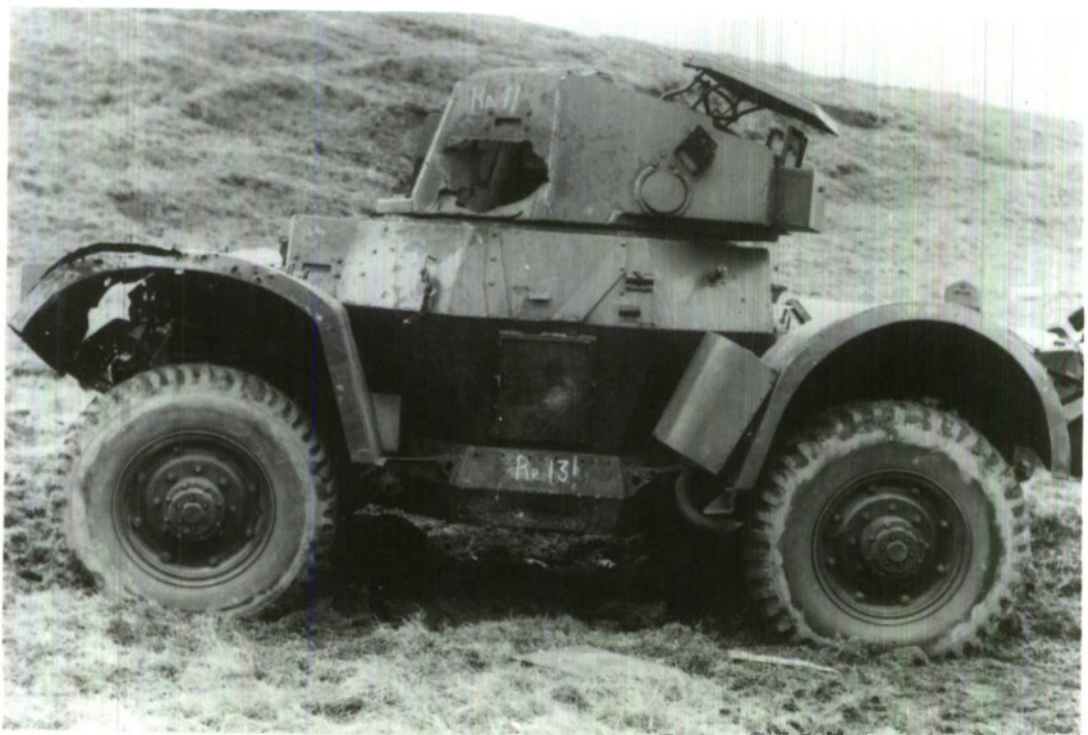
FIG. 4 NEAR MISS CLOSE TO CAR SIDE
