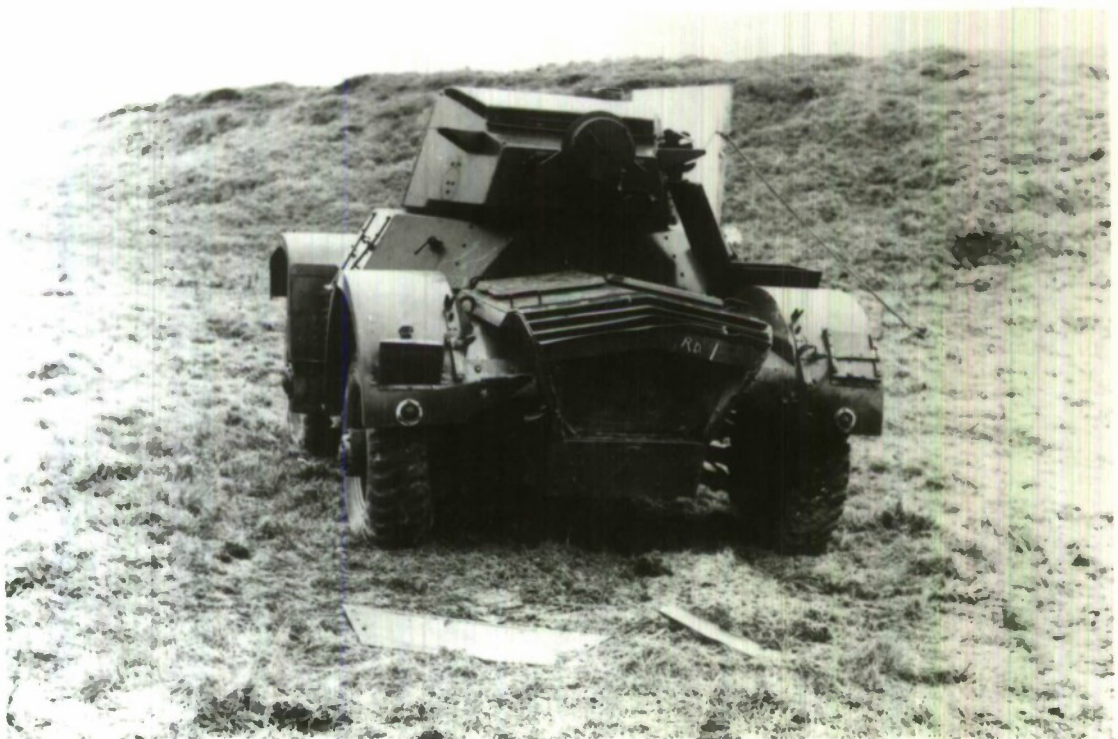
FIG. I NEAR MISS CLOSE TO THE ENGINE COMPARTMENT
