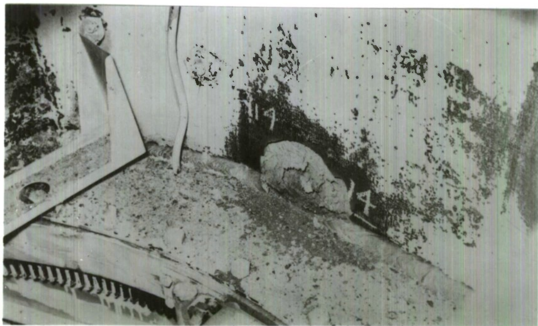
FIG. 25 DIRECT HIT ON PLATE OVER TURRET RING
