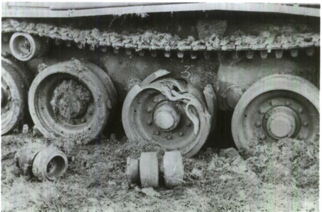
FIG. 16 DIRECT HIT ON CENTRE ROAD WHEEL RIM
