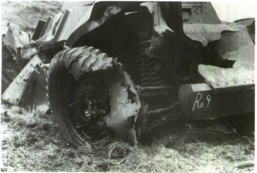
FIG. 8 DIRECT HIT ON WHEEL HUB
