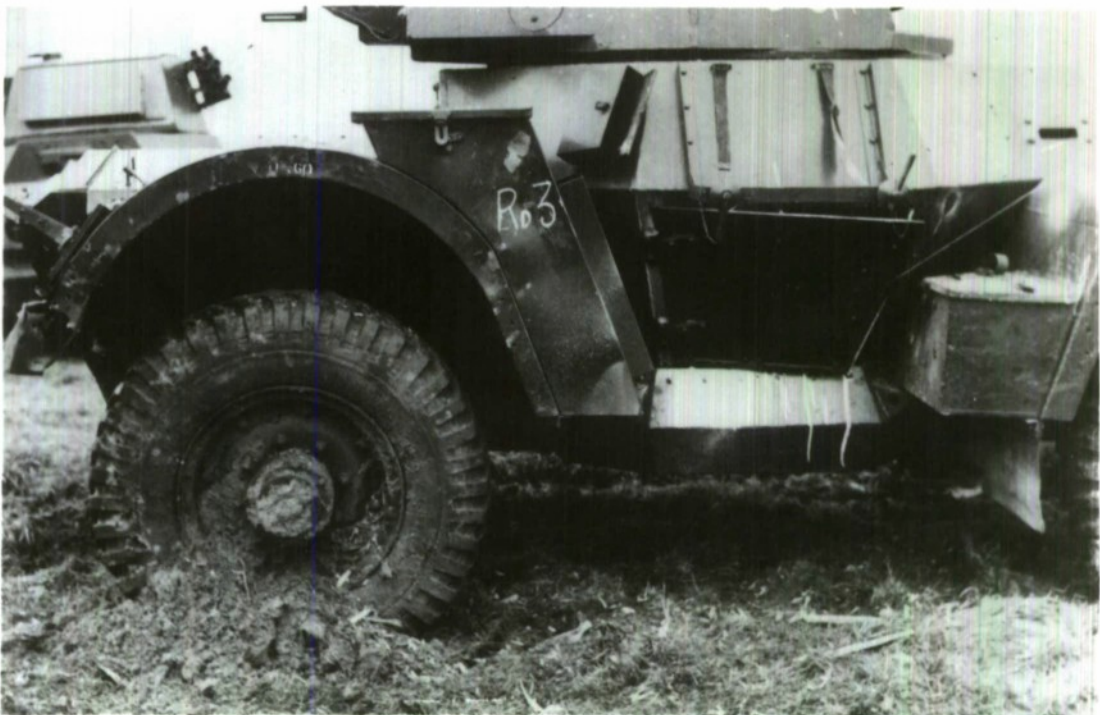
FIG. 3 NEAR MISS CLOSE TO A WHEEL
