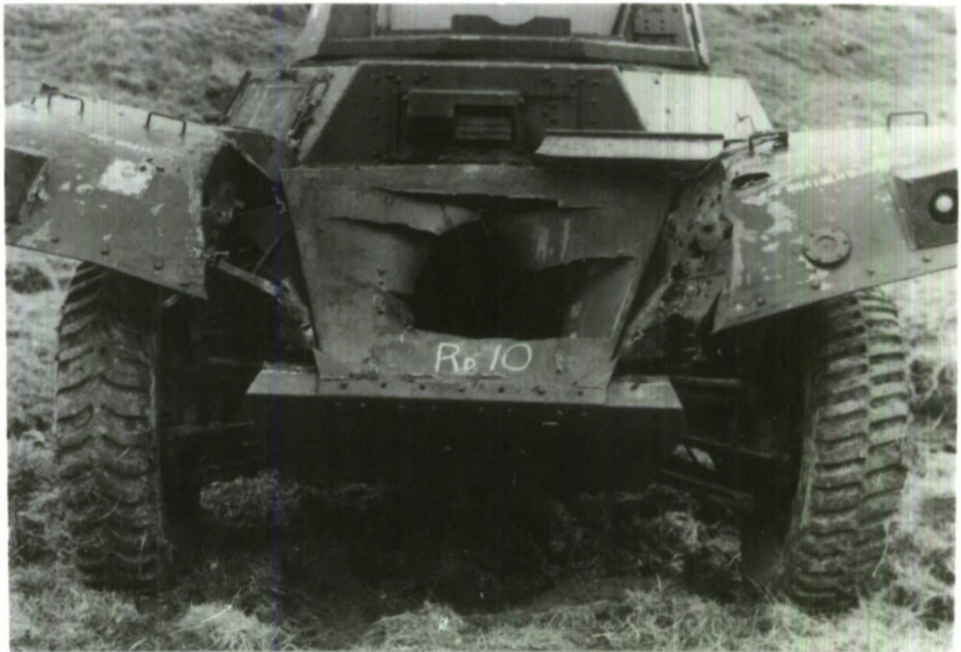
FIG. 11 DIRECT HIT ON CREW CONPARTMENT
