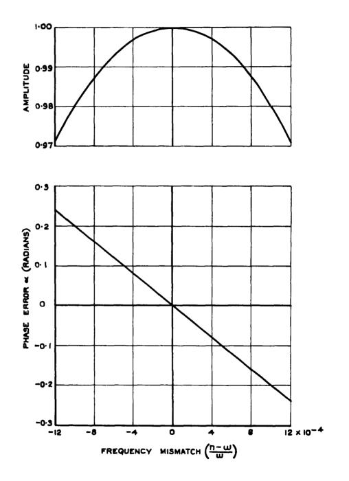
FIG.2.AMPLITUDE AND PHASE RESPONSE NEAR RESONANCE (Q = IOO)
