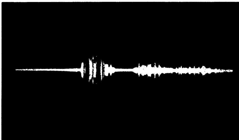
Fig. 2 - Backscatter amplitude at a 500 kc I-F on the vertical versus slant range in nautical miles on the horizontal. This picture was taken five minutes after launch.
