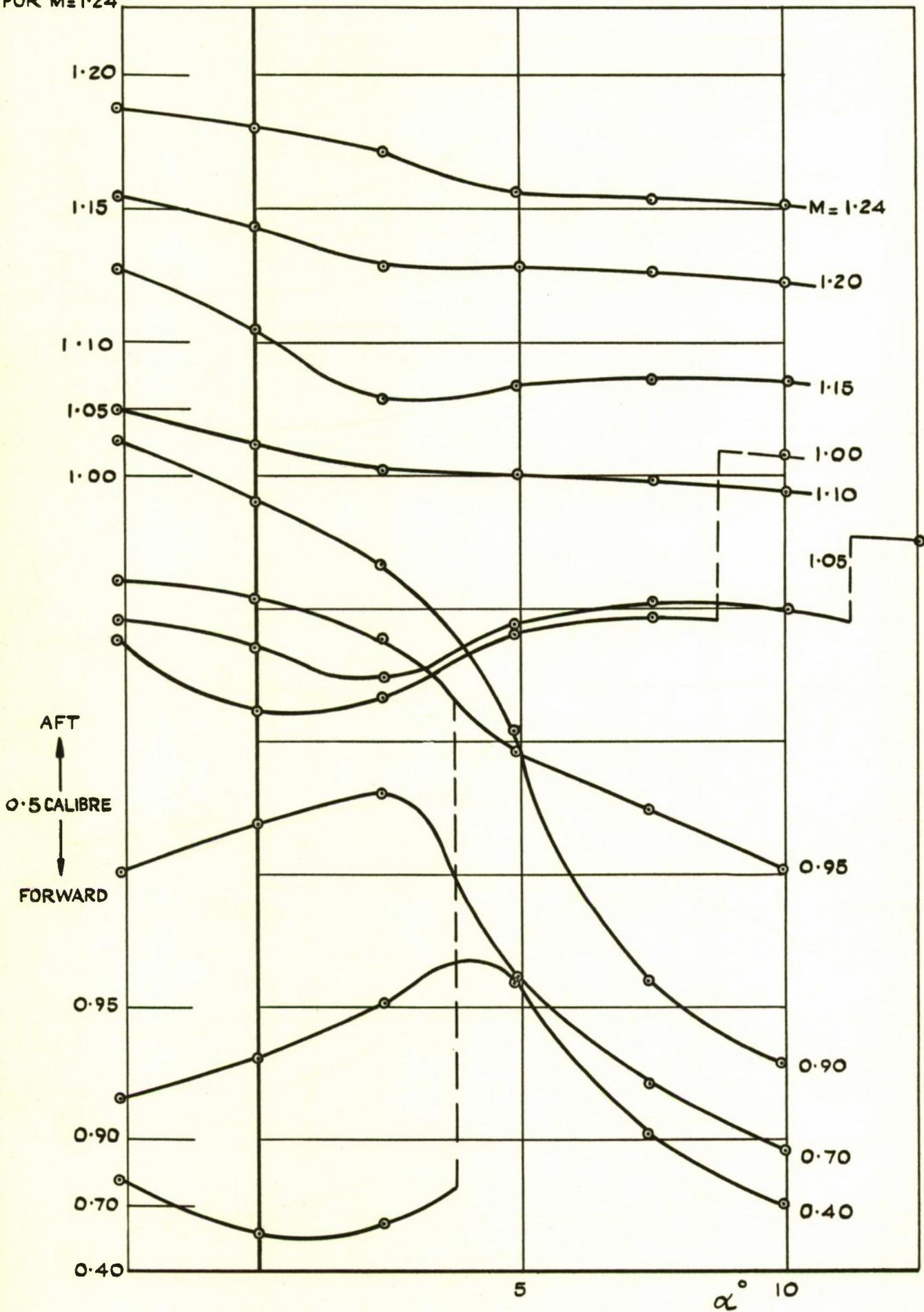
FIG. 14. POSITION OF CENTRE OF PRESSURE vs.  $\alpha$
