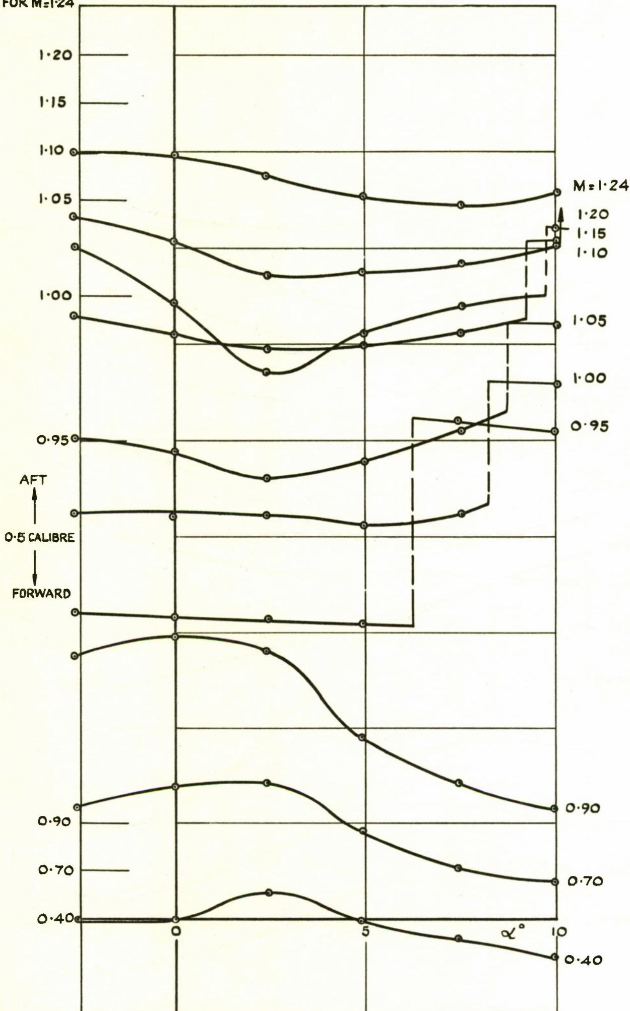
FIG. 12. POSITION OF CENTRE OF PRESSURE vs.  $\alpha$
