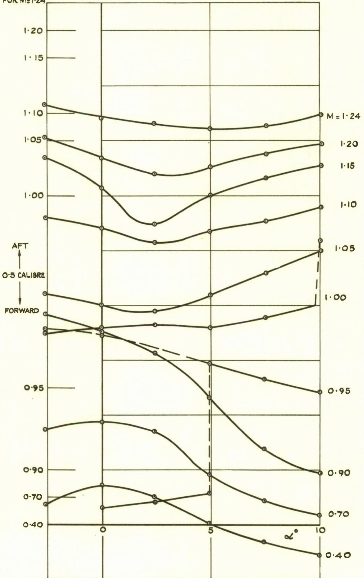
FIG. II. POSITION OF CENTRE OF PRESSURE vs.  $\alpha$
