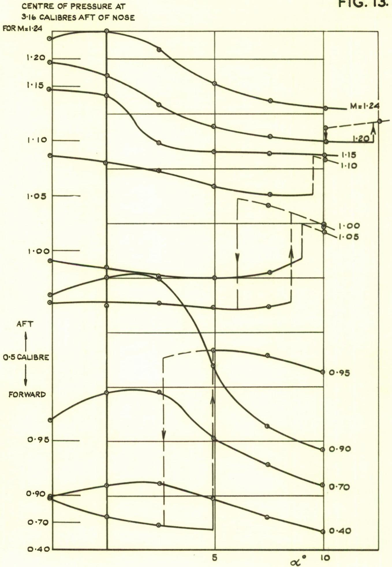
FIG. 13. POSITION OF CENTRE OF PRESSURE vs.  $\alpha$
