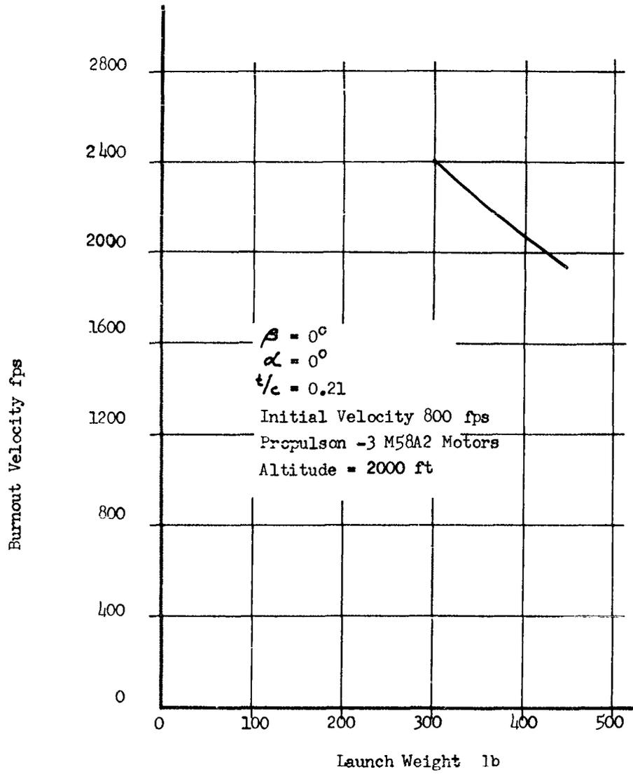
Figure 3.1 Variation of Burnout Velocity With Launch Weight
