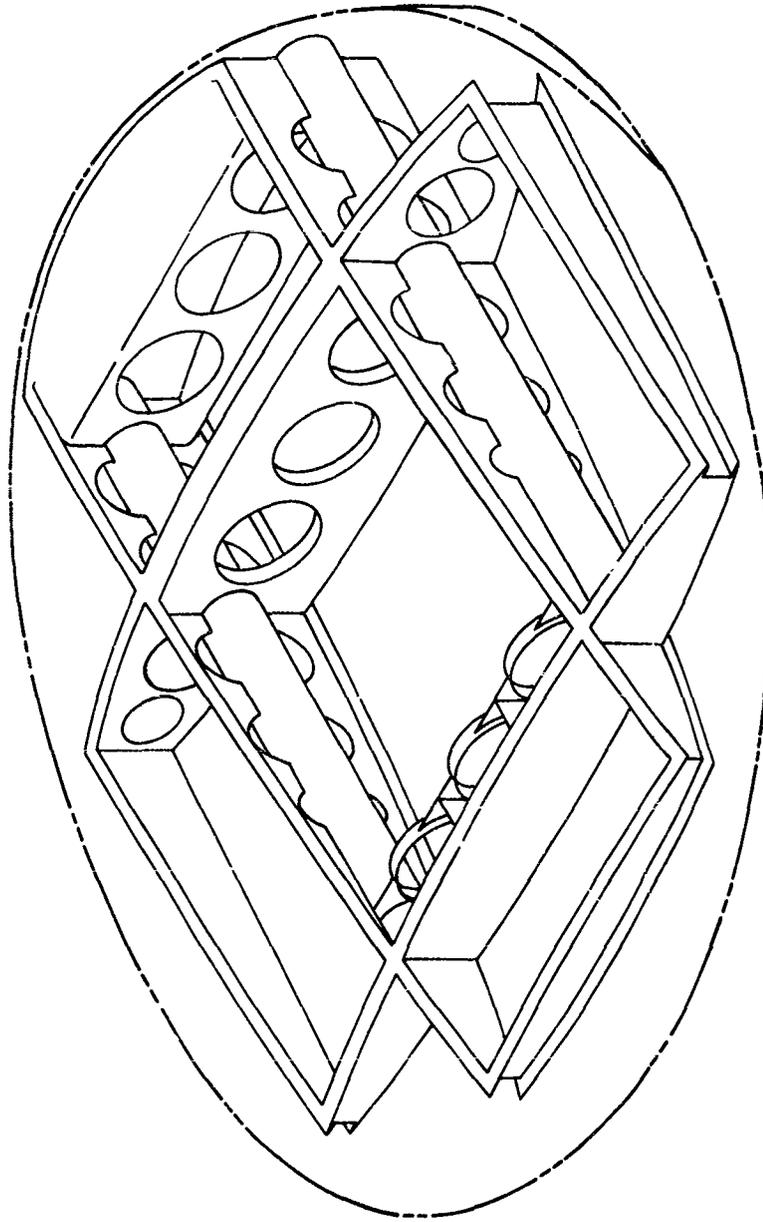
Figure 3.3 Main Structure Weldment
