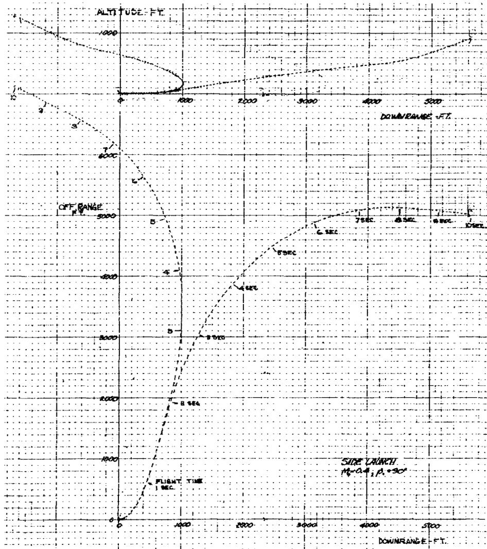
Figure 5.3 Side Launch Trajectories,  $M_0 = 0.4$ ,  $\beta_0 = 90^\circ$
