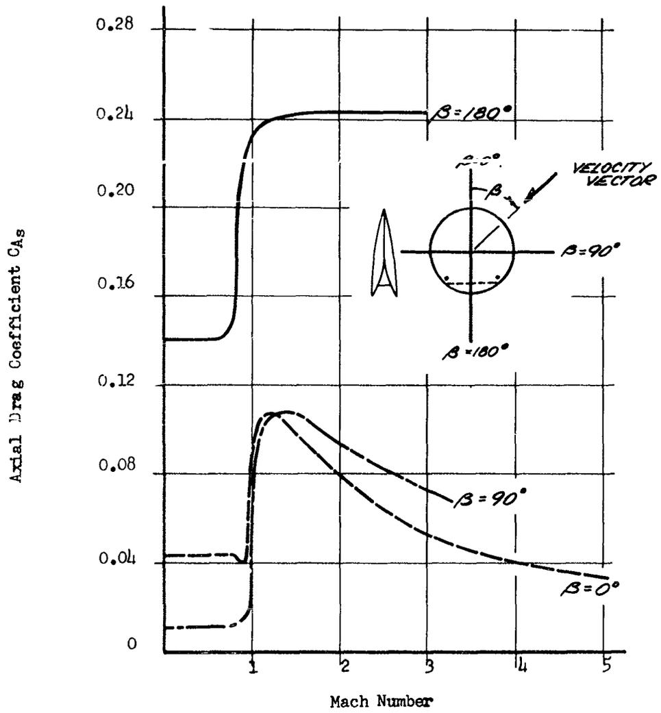
Figure 2.5 Variation of the Axial Drag Coefficient with Mach Number
