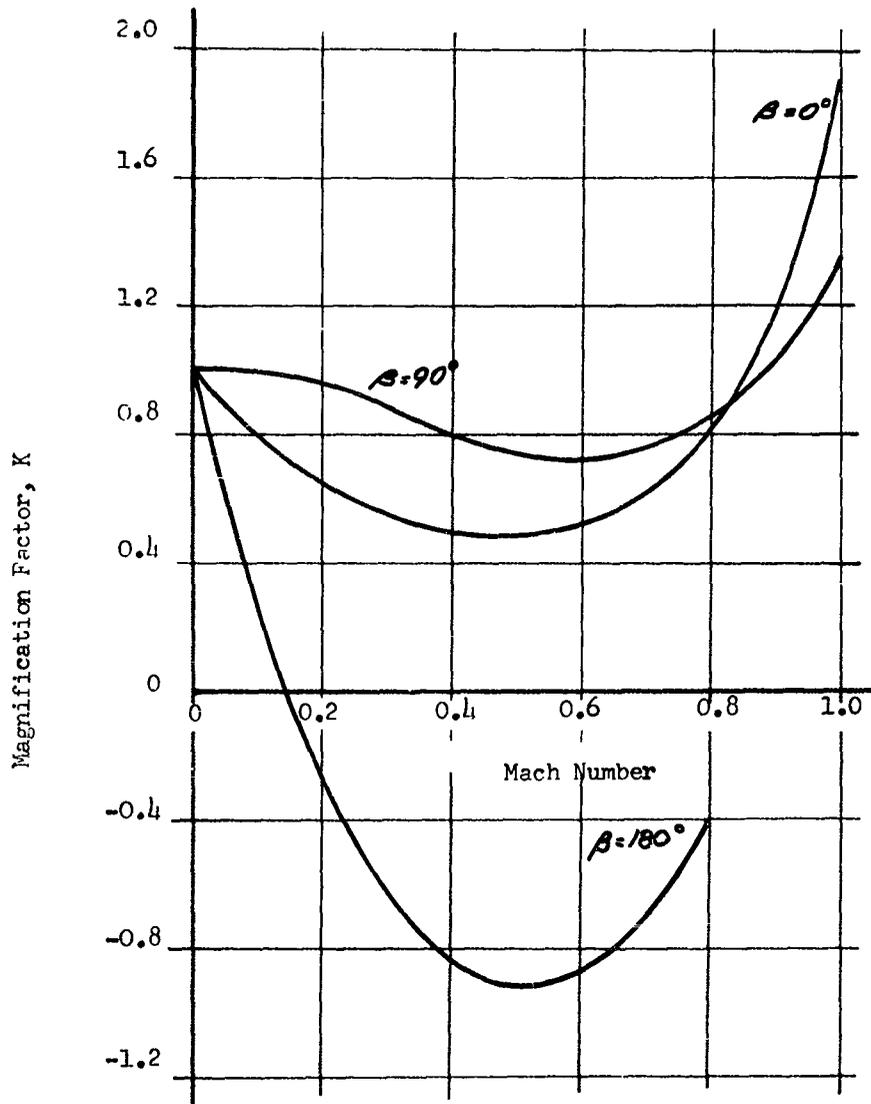
Figure 4.2 Variation of Magnification Factor With Mach Number
