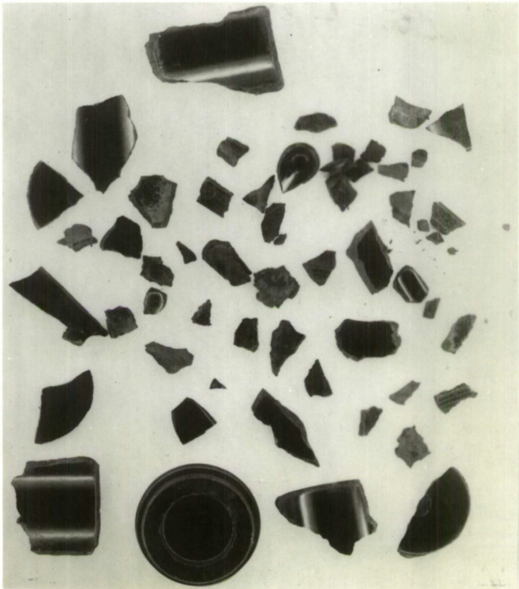
FIG. 2 FRAGMENTATION FROM CARTRIDGE, COOLER, 1.5 INCH, TYPE 2 (APPROX. FULL SIZE)
