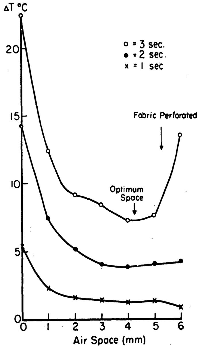
Figure 6. Temperature rise within simulated skin vs. thickness of air space between two layers of 3 oz/yd<sup>2</sup> fabric.
