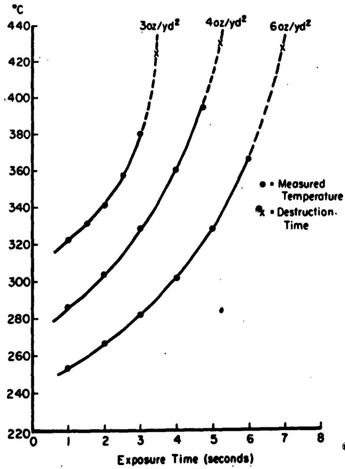
Figure 4. Radiometric measurement of destruction temperature.
