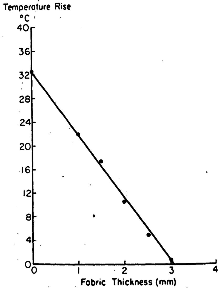
Figure 5. Temperature rise within simulated skin vs. thickness of fabric applied.
