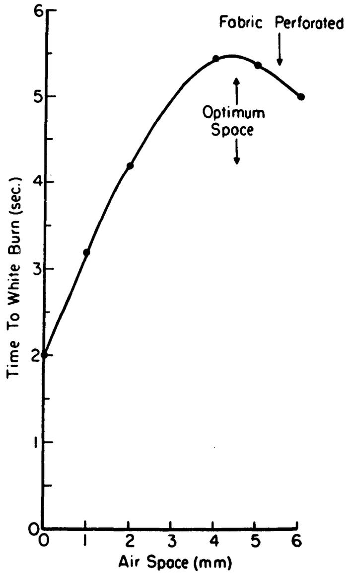
Figure 7. Exposure time productive of white burn in anaesthetized, depilated rat vs. thickness of air space between two layers of 3 oz/yd<sup>2</sup> fabric.
