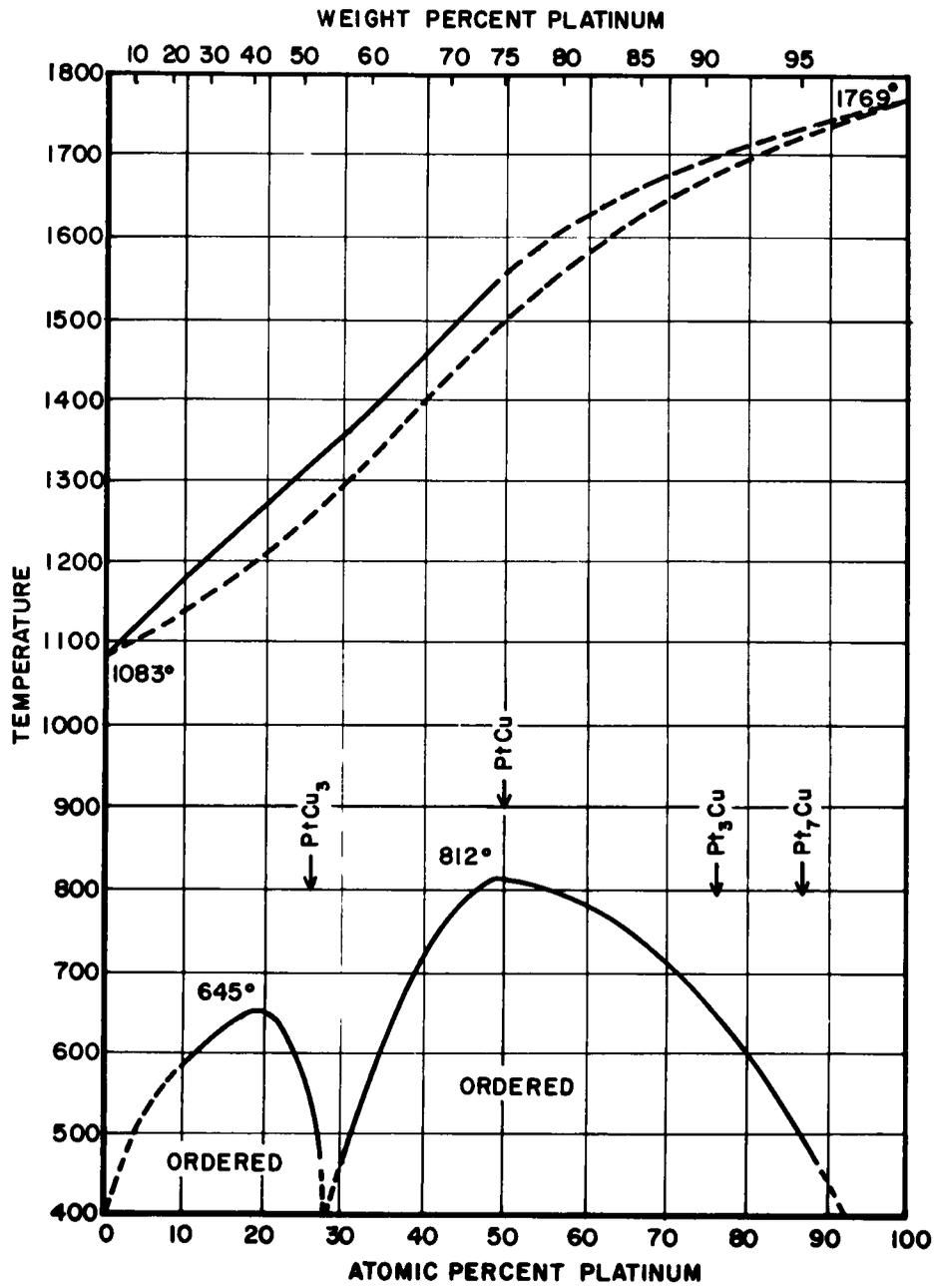
Figure 1. Cu-Pt Phase Diagram
