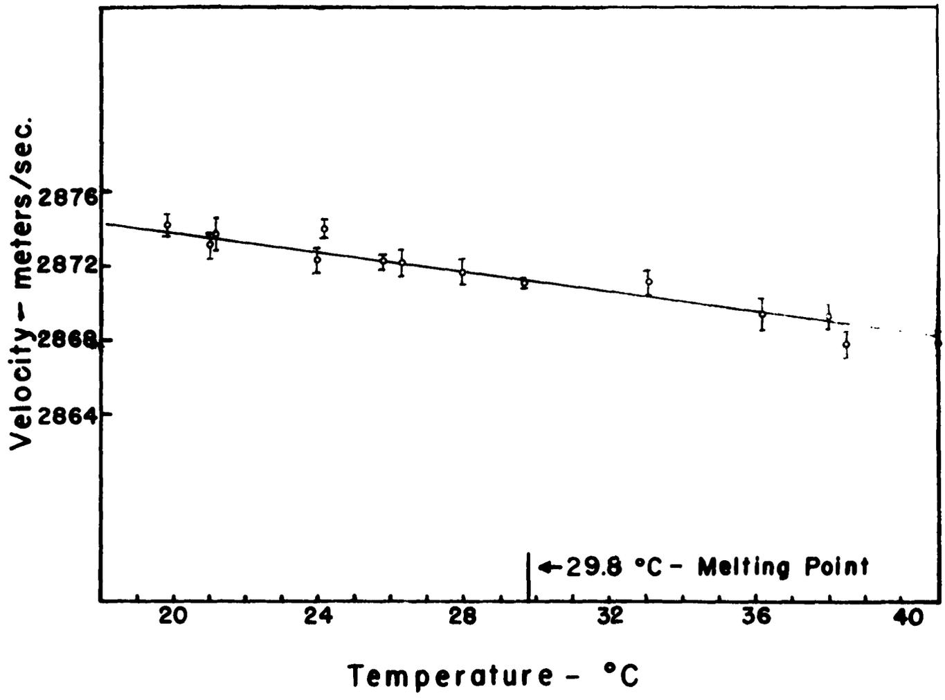
Fig. 3 Velocity versus Temperature for Liquid Gallium.
