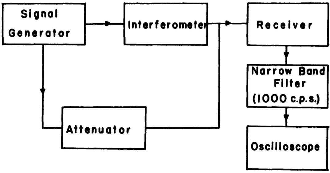
**Fig. 2 Block Diagram of Velocity Measurement System.**
