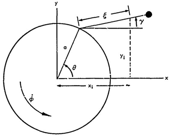
Figure 6 - Coordinate system for distributed weight of wire
