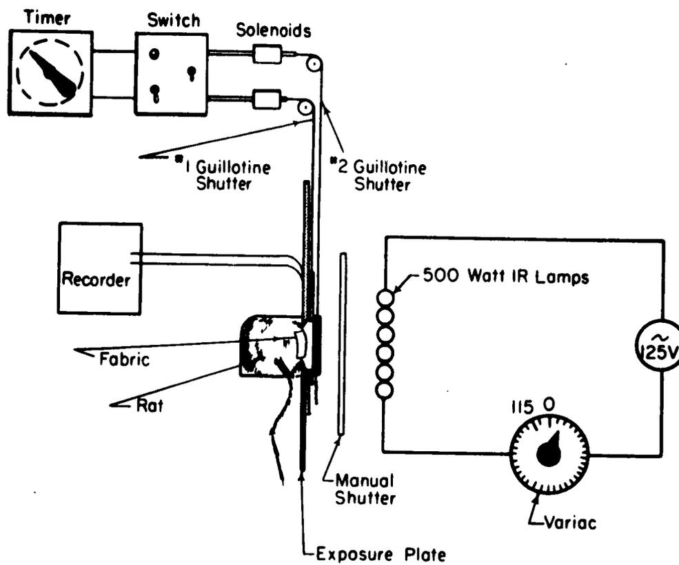
Figure 1. Thermal irradiation apparatus.
