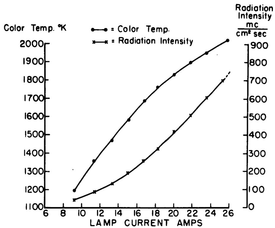
Figure 2. Color temperature and irradiance of infrared quartz lamp source.
