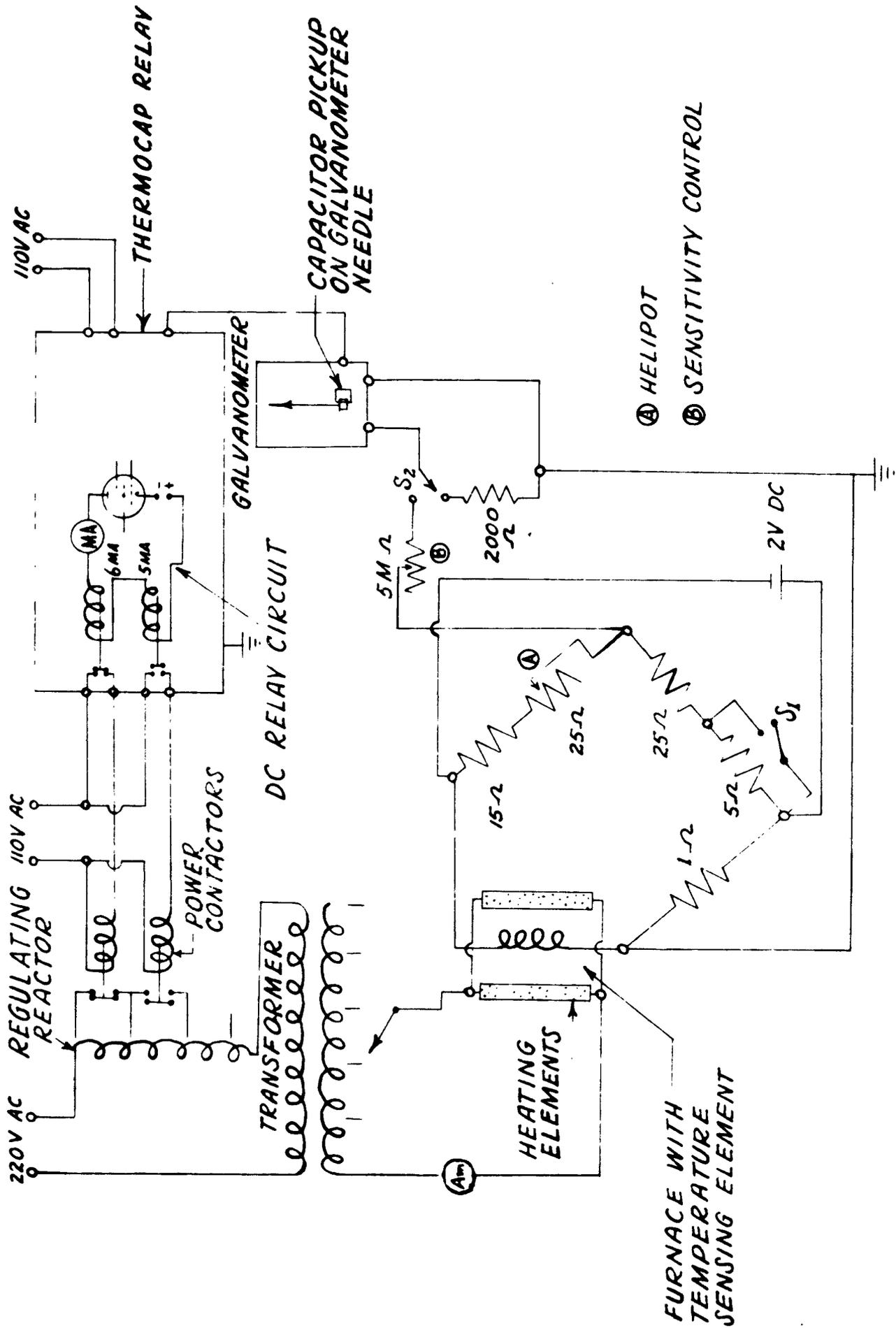
FIG. 2. SCHEMATIC DRAWING OF TEMPERATURE CONTROL CIRCUIT
