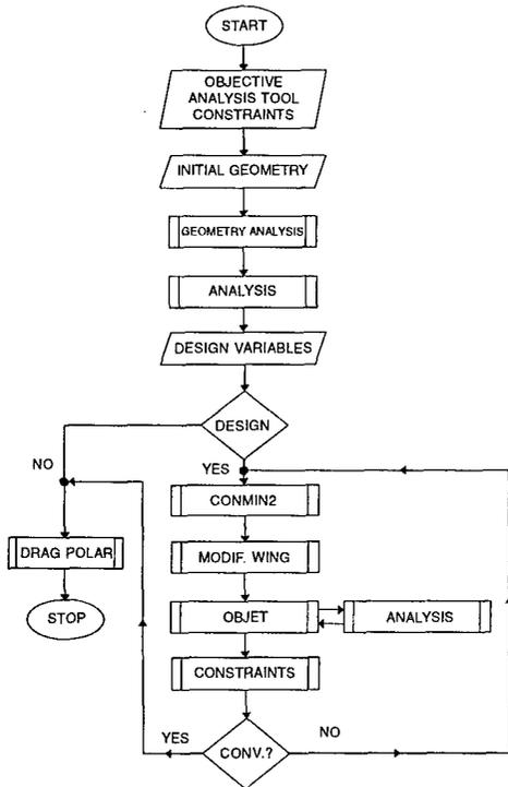
Figure 1: Flow chart for the aerodynamic optimization procedure
