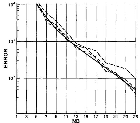
Figure 3: Bèzier fitting error for different airfoils
