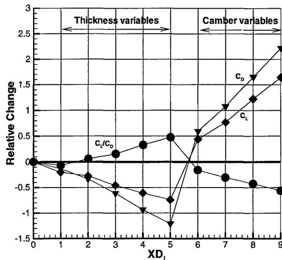
Figure 7: Sensitivity analysis for the subsonic case
