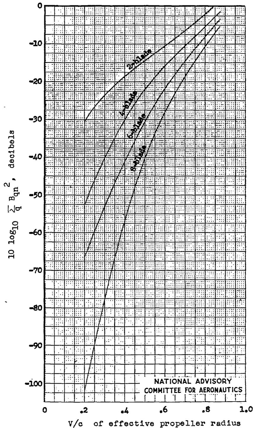
Figure 3.- Function  $10 \log_{10} \sum B_{qn}^2$  for various numbers of propeller blades.
