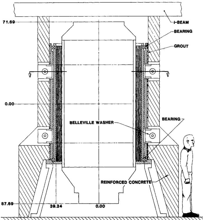
Fig. 6. 10-MJ ARFC flashlamp driver in torque frame
