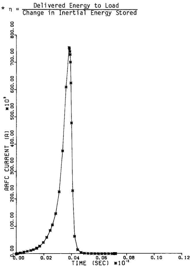
Fig. 4. Computed discharge current waveform
