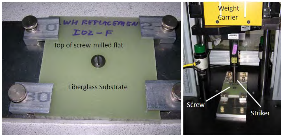
Figure 13. Close ups of a screw prepared for impact testing. The drop weight impact tester is an Instron Dynatup model 8100. Instrumentation in the striker holder measures the force of impact.
