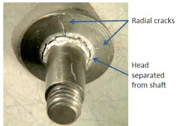
Figure 15. Example of severe damage inflicted by high force impact, showing circumferential cracking and radial cracking.
