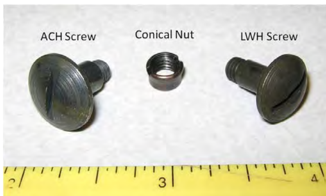
Figure 1. Helmet hardware tested by NRL in this study. Both ACH and LWH use the same nuts.
