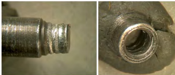
Figure 8. Stripped threads of an LWH screw. The nut (on the right) threads are intact, and pieces of the screw threads are visible inside the nut
