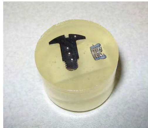
Figure 3. Example of cross-sectioned screw (ACH in this example) and nut mounted in plastic and polished. The marks on the surface of the screw are Rockwell hardness indentations.
