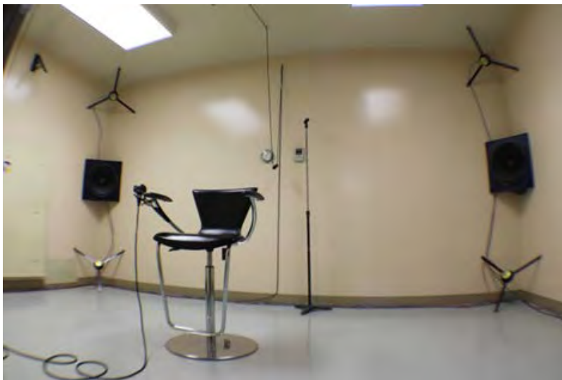
Figure 4. Facility used for measurement of continuous noise attenuation
