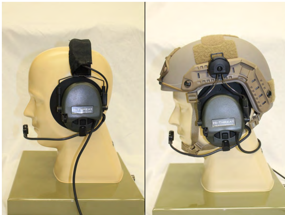
Figure 2. TEA HI Threat headset with and without Ops-Core ACH and the ARC HTH System
