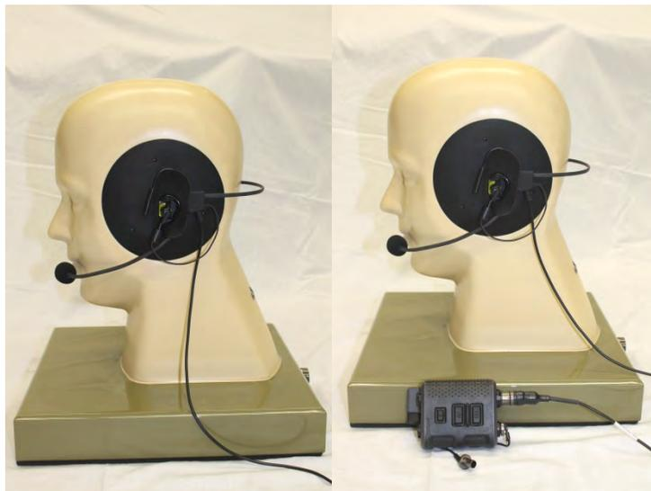
Figure 2. OTTO Hurricane Headset (left) and Invisio V60 with OTTO Hurricane headset (right)
