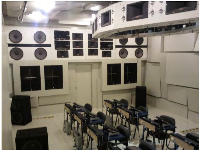
Figure 14. AFRL's VOCRES facility used to measure speech intelligibility performance
