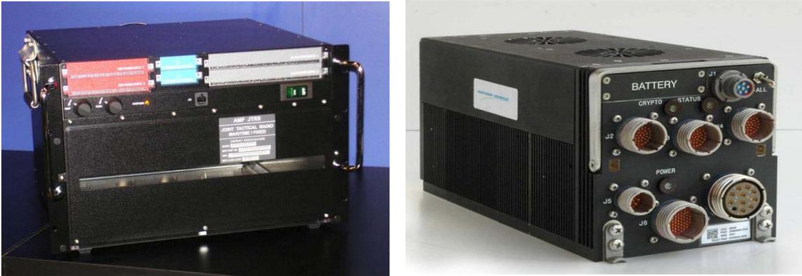
**Figure 9. JTRS Airborne Maritime and Fixed Station Radios: Maritime Fixed JTR (left) and Small Airborne JTR (right)**
