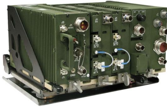
**Figure 12. JTRS Ground Mobile Radio**
