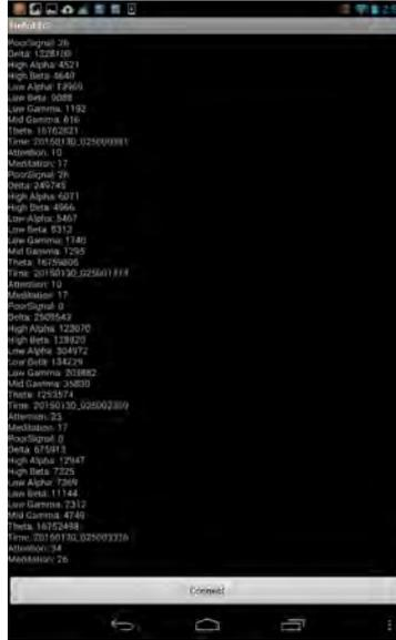
Figure 4: Example UI of HelloEEG. Part 1 represents the signal strength Part 2 is the sampled data of 8 wave ranges. Part 3 is the timestamp. Part 4 is the attention and meditation level based on NeuroSky algorithm.
