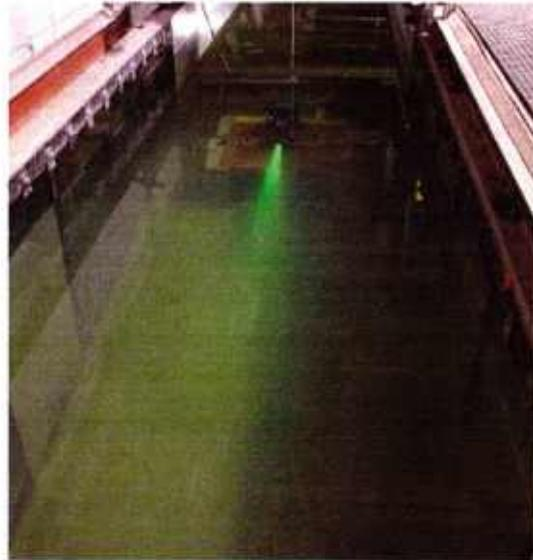
(b) LUCIE submerged in the flume imaging the test board
