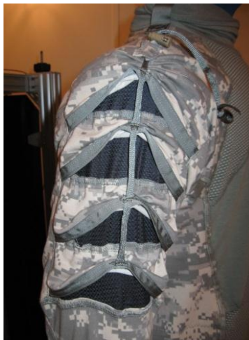
Figure 1 Prototype CB Protective Garment with Ventilation Concept on Upper Arm (Nett Warrior prototype, developed by NSRDEC team).
