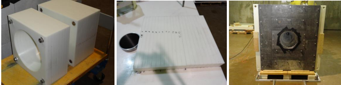
Figure 2: The collimator assembly during construction (left), installed in the moderator (center), and covered with lead sheeting to shield the image plane (right).
