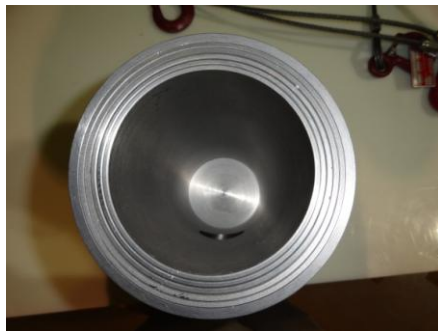
Figure 1: Low-carbon steel insert used to slow the high-energy D-T neutrons over a shortened distance.
