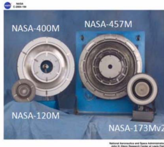
Figure 1 A selection of NASA Hall Thrusters 25 .
