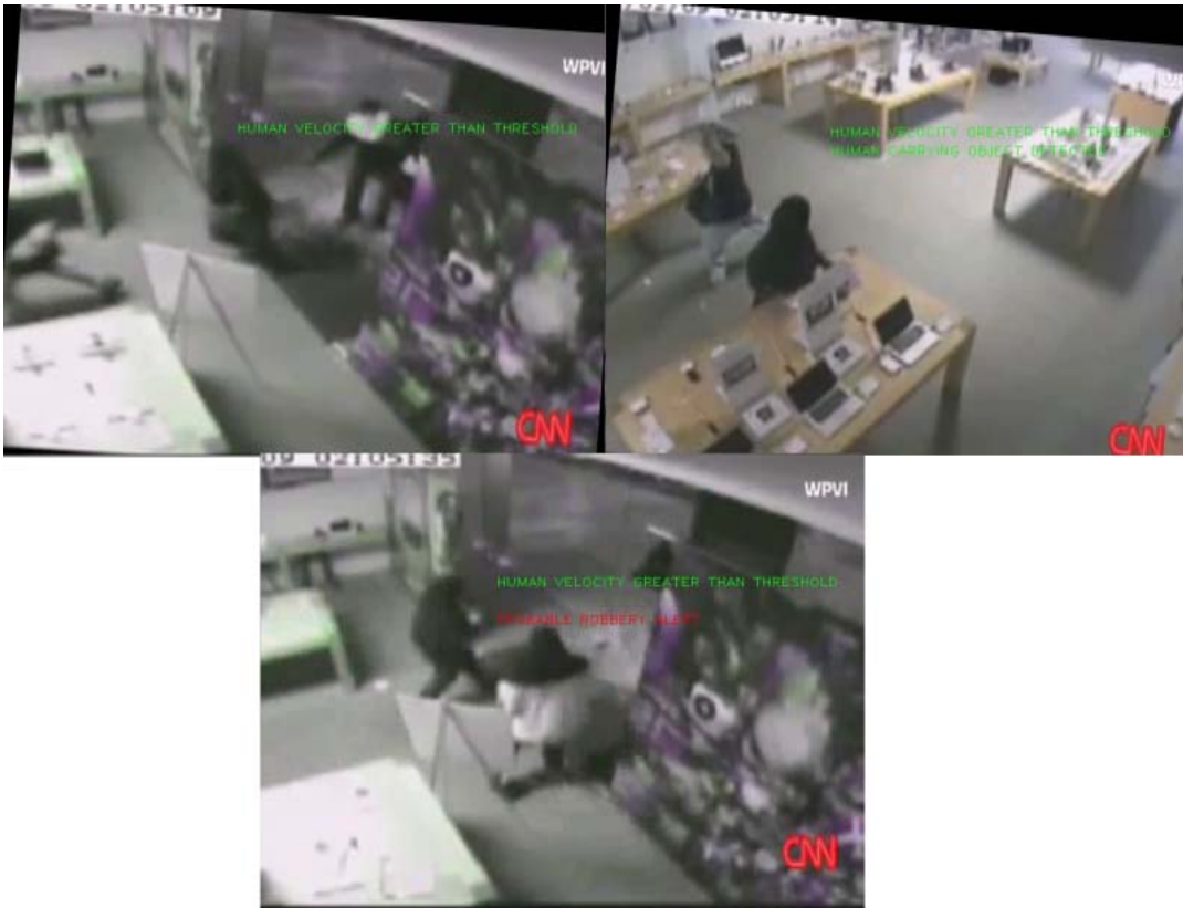
Fig 3. Human velocity greater than threshold and Human carrying object detected inside store, so, probable burglary alert
