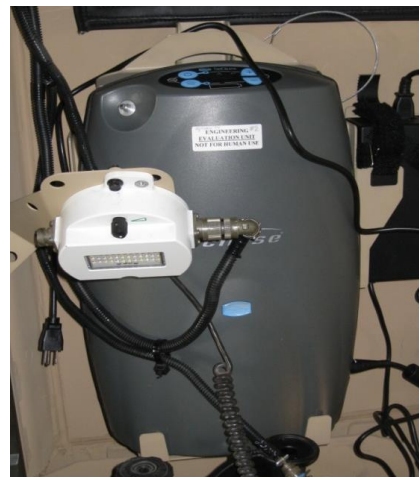
Figure 4b: Oxygen concentrator in an MWRAP.
