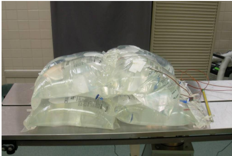
Figure 3: Arrangement of the PrismaSate® bags to develop the fluid model used in this study.
