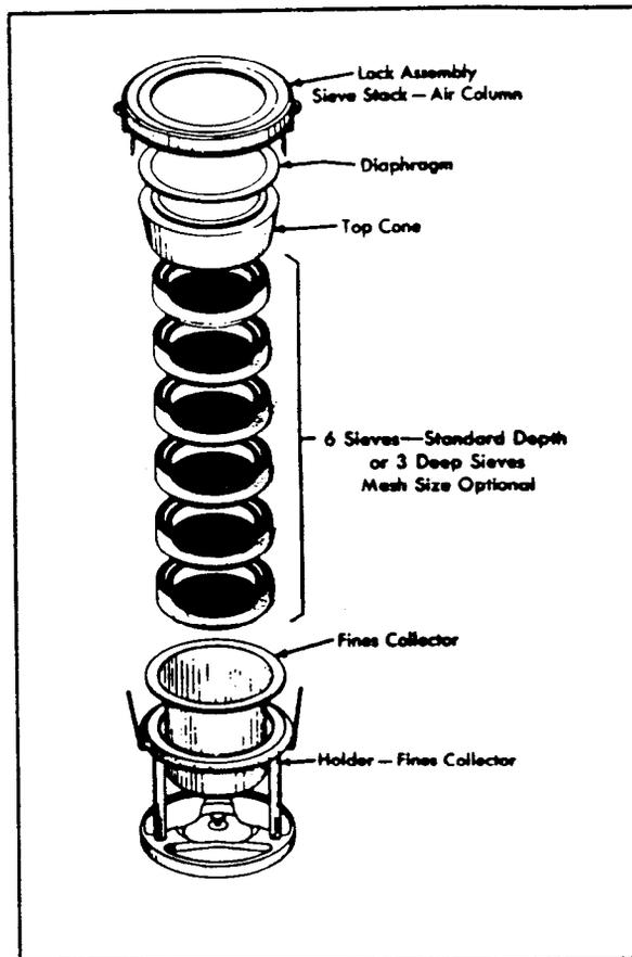
Figure 1. Sieve Stack Assembly
