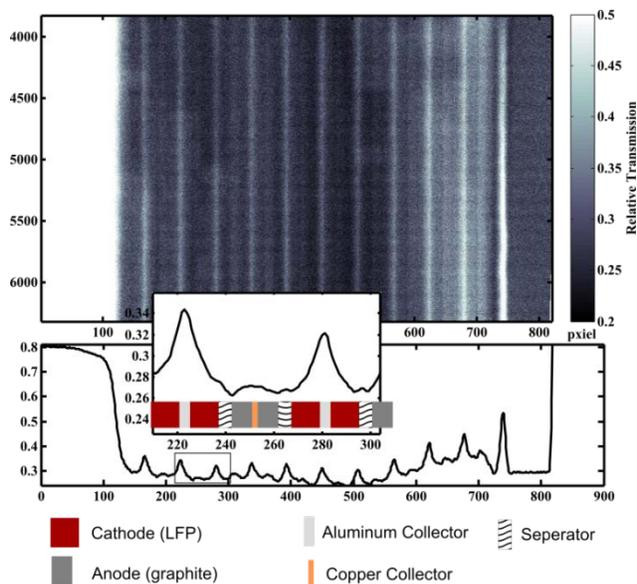
Figure 4: Neutron transmission image of the battery and corresponding line profile from averaging along the y-axis in the image. The peaks in the line profile are caused by the aluminum current collectors which have significantly lower neutron attenuation than other materials present in the battery.
