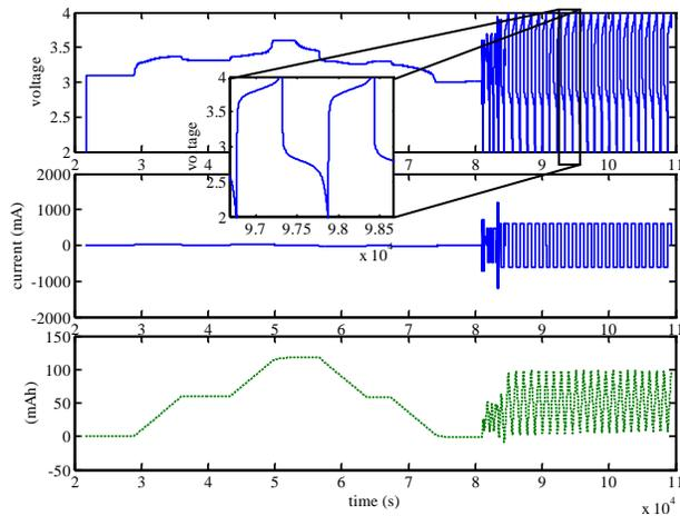
Figure 6: Measured voltage (top), applied current (middle), and stored charge (bottom) for the slow and fast cycling of Sample A. At the 5C rate approximately 75% of the total capacity was available when cycling between 2 and 4V.
