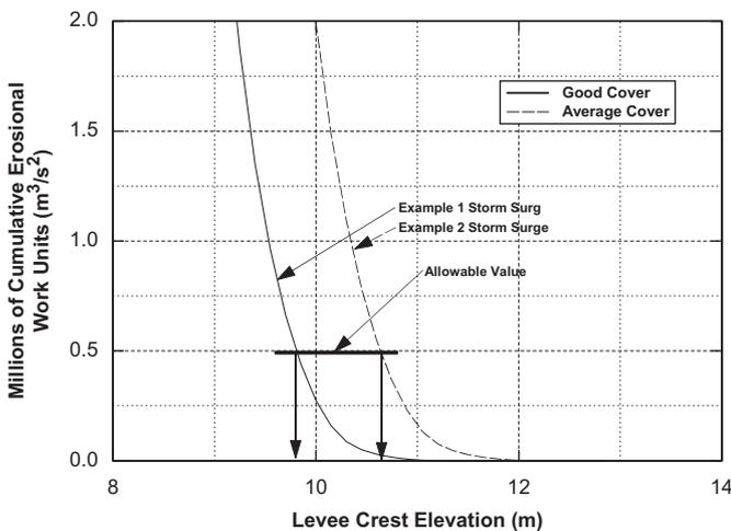
Fig. 13. Effect of storm surge hydrographs: comparison of cumulative erosional work unit results for Examples 1 and 2 and associated levee crest elevations. Good quality grass cover.
