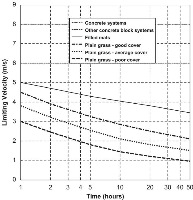
Fig. 3. Combinations of (velocities, durations) for acceptable erosion of various coverings due to steady overtopping (Hewlett et al., 1987) as reported in Hughes (2007).
