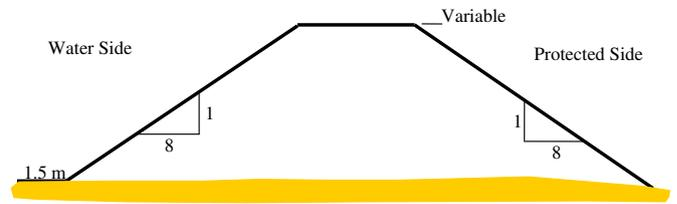
Fig. 7. Example levee cross-section.
