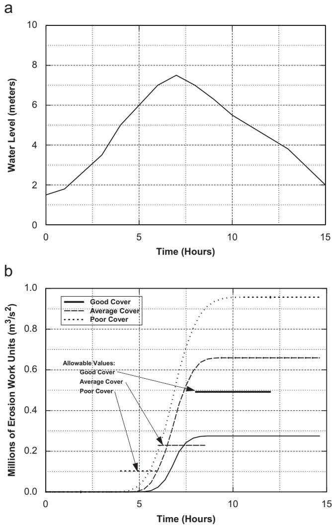
Fig. 9. Time variation of erosion work units for storm surge of Example 1 and three grass cover qualities. Levee crest elevation = 10 m for this case. (a) Time variation of total storm surge for Example 1 and (b) time variation of cumulative erosional work units for Example 1.
