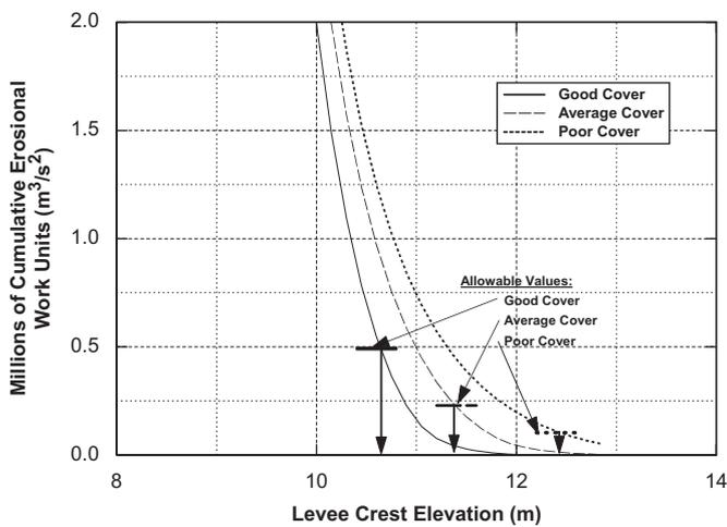
Fig. 12. Example 2: variation of cumulative erosional work units vs. levee crest elevation.
