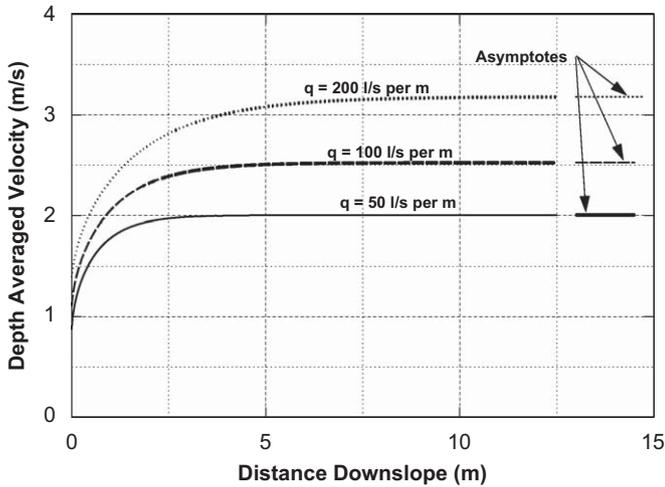
Fig. 2. Variation of depth averaged velocity vs. distance for three unit discharge values. Note these three cases commenced with 90% of critical depth at the landward side of the levee crest. Land side slope = 1:6.
