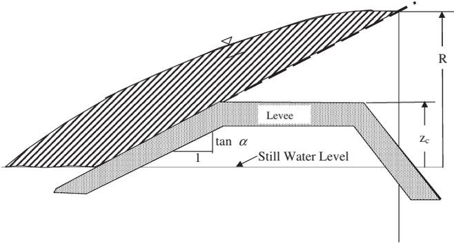
Fig. 5. Definition sketch for potential wave runup.
