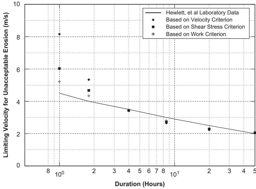
Fig. 4. Comparison of fits of three erosion indices results to Hewlett's measurements for "Plain Grass-Good Cover".
