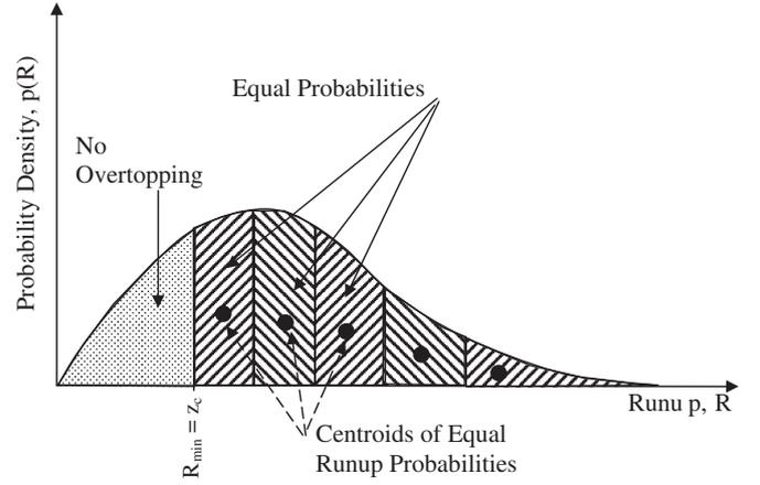
Fig. 6. Schematization of runup probability distribution showing the portion of the distribution which contributes to overtopping.
