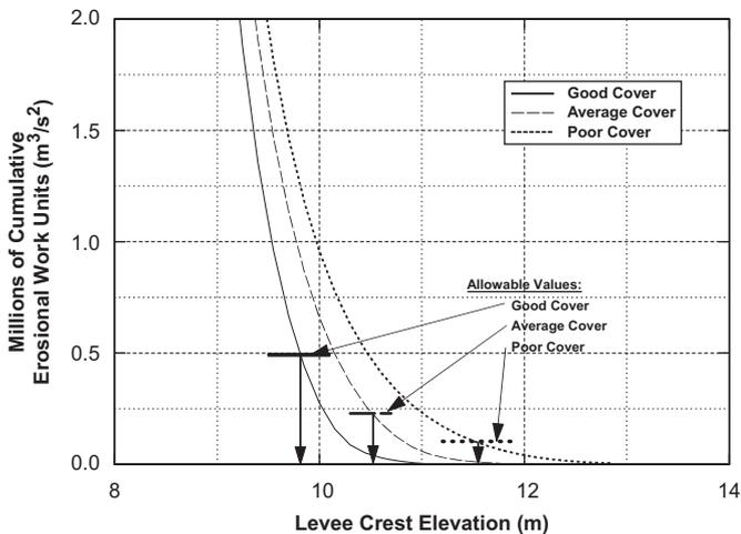
Fig. 10. Example 1: variation of erosional work units vs. levee crest elevation.
