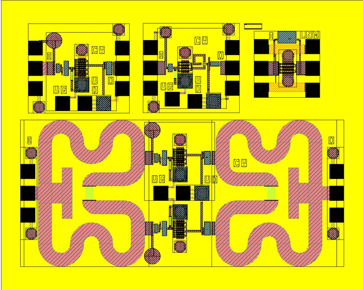
Figure 2. CKT2 30-GHz Harmonic two way combiner PA 2.5 mm x 2 mm.
