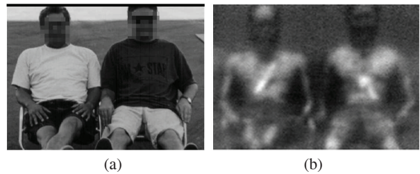
Fig. 1. Millimeter wave imaging through clothing. (a) Visible image of the scene. (b) Image produced using a 94-GHz imaging system.
