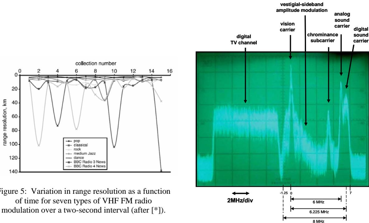
Figure 5: Variation in range resolution as a function of time for seven types of VHF FM radio modulation over a two-second interval (after [\*]).
