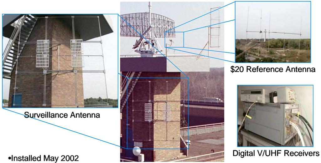
Figure 13: FM radio-based bistatic radar, showing surveillance and direct signal antennas and digital receivers [34].
