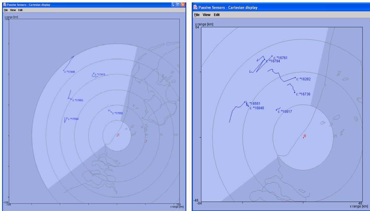
Figure 14: Examples of tracks of aircraft over the North Sea obtained with PBR system located at The Hague [34].
