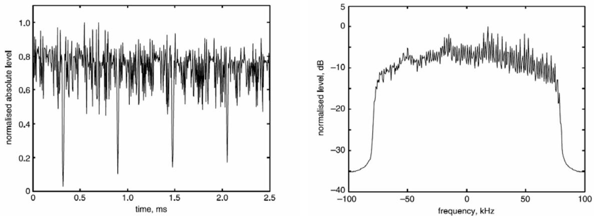
Figure 8: (a) time-domain representation of part of one TDMA-modulated carrier of a GSM signal, showing the 577  $\mu$ s slots; (b) frequency-domain representation, showing the 200 kHz channel (after Tan et al. [49]).
