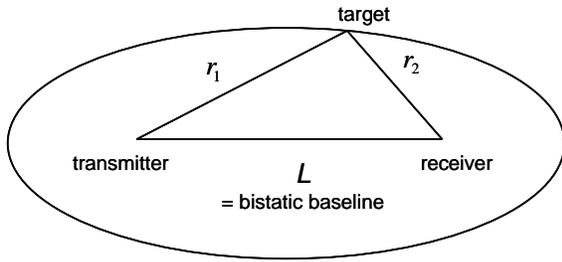
Figure 1: Bistatic geometry [35].
