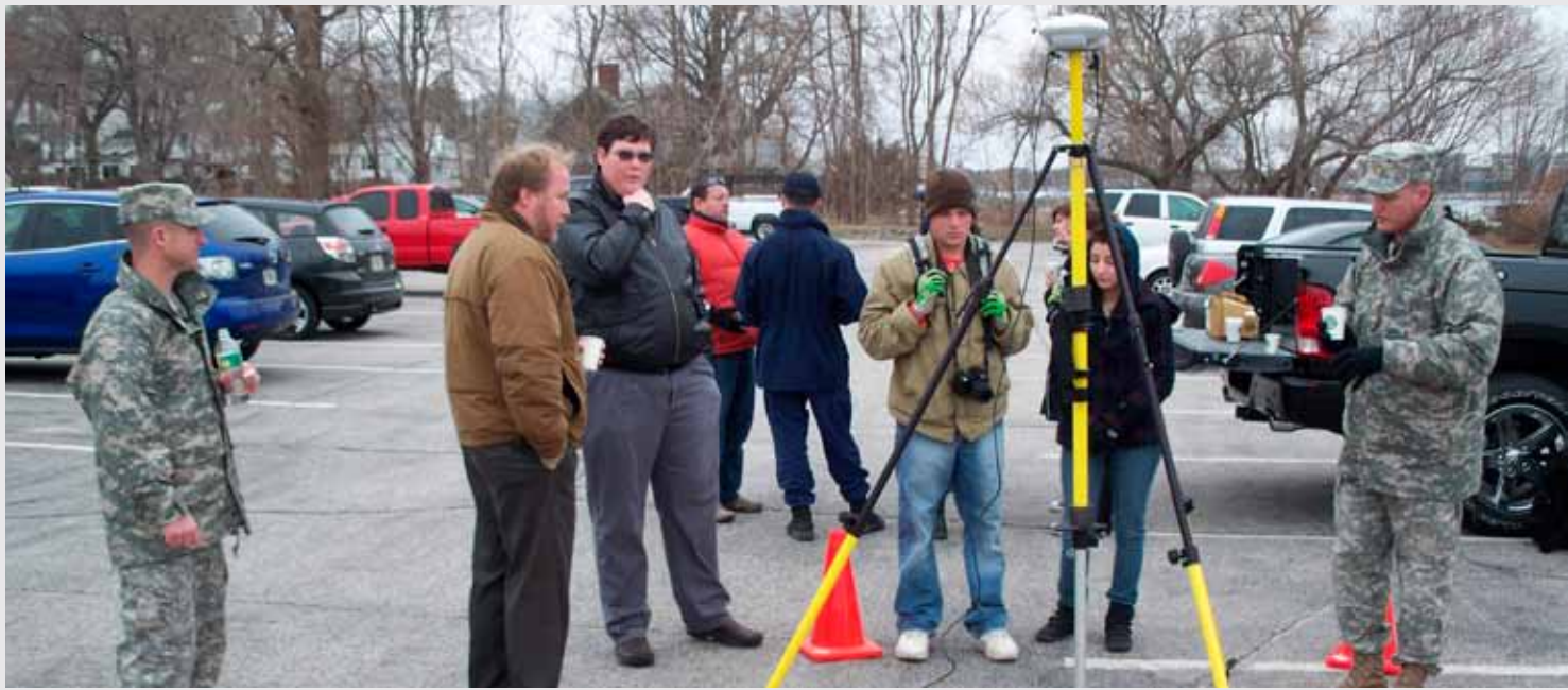
A GPS base station setup by West Point's Surveying class for Real Time Kinematic Surveying. This project involved West Point, the United States Coast Guard Academy, and Mitchell College students. There were three different projects involved in this effort, mapping and removal of invasive plant species, temporal change of the beach, and a survey stake out for the design and construction of a boardwalk civil engineering project. From left to right - MAJ Hannon Didier, Mr. David Shirley (Keystone Precision Instruments), Mitchell College Students, and MAJ Wright in ACU's. U.S. Army Photo
