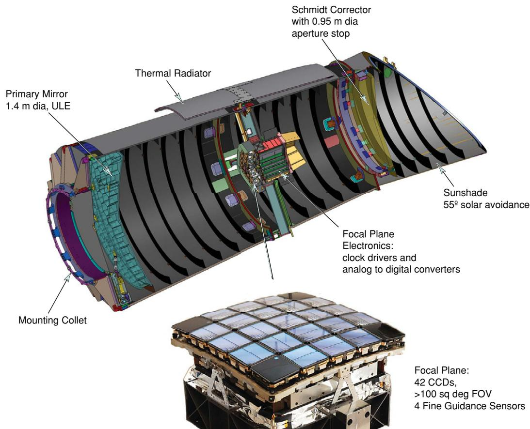
**Figure 2.** Cross-sectional view of the photometer and inset of the focal plane. The overall height with the sunshade is 4.3 m. The spacecraft (not shown) is a hexagonal structure 0.8 m high that surrounds the base of the photometer.
