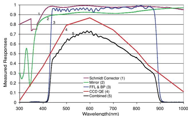
**Figure 1.** Spectral response curves. An average value is shown for the 21 FFLs and the BP filters, which are multi-layer coatings on the back of the sapphire FFLs. The CCD QE is the average from all 42 CCDs. The combined response curve also includes a 4% loss for contamination
