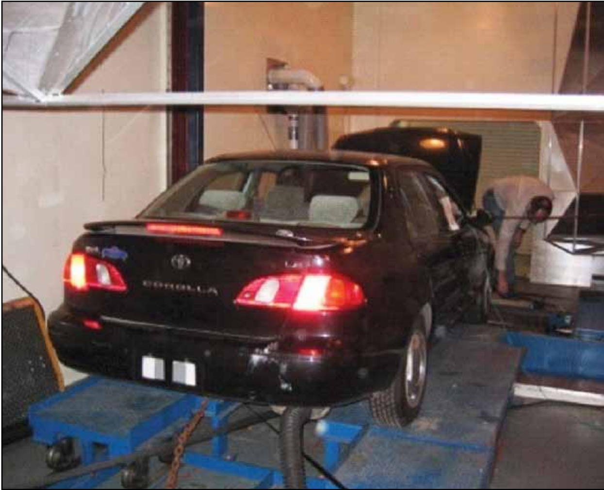
Figure 2. Vehicle on a Dynamometer in the NSWCCD Reverberation Chamber
