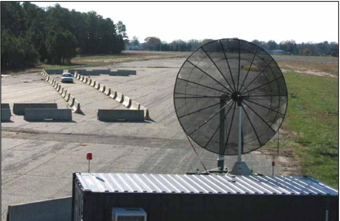
Figure 3. Multifrequency RF Vehicle-Stopper (RFVS) System
