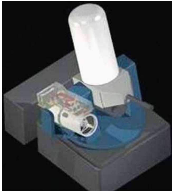
Figure 1. LaWS Mounted on CIWS
