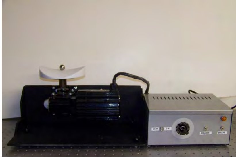
Figure 7. Side view of the apparatus used for demonstration of the trapping potential. The saddle surface has a diameter of 15cm, and the steel ball is 1.9cm in diameter.
