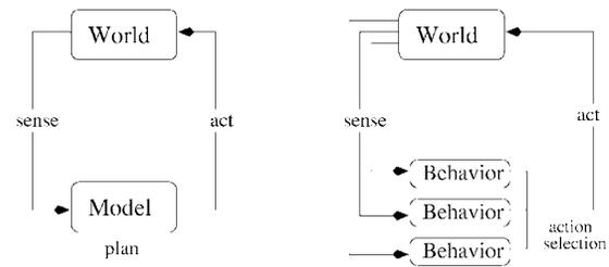
**Figure 1.** Behavior-based control differs from conventional control by composing overall vehicle behavior into distinct modules that are developed and operate largely in isolation, and coordinated through an action selection mechanism. In this case, action selection is in the form of a new multiobjective optimization technique to overcome known difficulties associated with behavior-based control.
