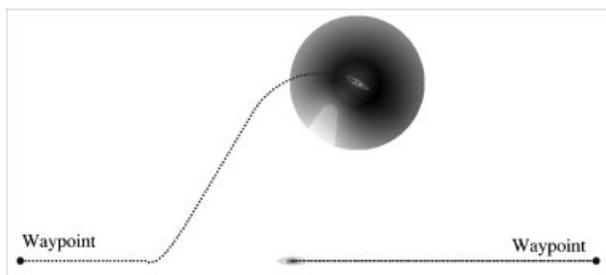
**Figure 5.** In simulation, the lefthand vehicle is guided by a waypoint and collision avoidance behavior to the point on the right. (Note this vehicle passes to the opposite side as would be prescribed by the COLREGS. Compare this trajectory with Figure 11.) The righthand vehicle is executing a waypoint behavior with no collision avoidance to the waypoint on the left. The function rendered represents the addition of the two objective functions at that point in time.
