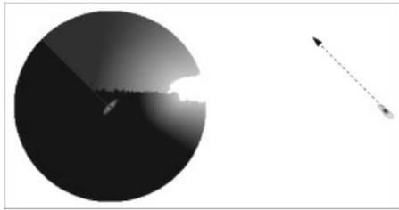
**Figure 9.** The crossing behavior produces objective functions based in part on the closest point of approach for a candidate maneuver and in part on a preference maneuvers that do not cross ahead of the other vessel. Darker colors represent more favorable actions, and larger radii on the plot indicate higher candidate speeds. [Compare with Figure 4(b).]
