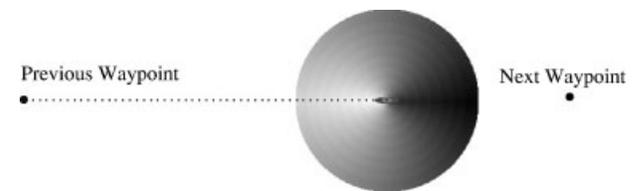
**Figure 6.** The objective function produced for the waypoint behavior rates decisions higher that bring the vehicle closer to the next waypoint and do not add detour distance. The utility drops linearly. This is a radial plot over heading and velocity. Darker shades represent higher utility. Typically about 600 linear pieces are used to represent this function.
