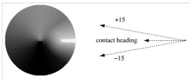
**Figure 7.** The head-on behavior produces objective functions based in part on the closest point of approach for a candidate maneuver and in part on a preference for starboard maneuvers passing the contact on the port side. Darker colors represent more favorable actions, and larger radii on the plot indicate higher candidate speeds. Compare against Figure 4(b) where maneuvers to either side of the contact are nearly equal in preference.
