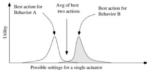
**Figure 3.** The average of the best action produced by two behaviors may have poor value for *both* behaviors. The chooser of the action is oblivious to the error since the behaviors output a single preferred action and do not communicate the underlying effectiveness of their alternatives, rendered here only for illustration. In this case, interests being pursued by the two behaviors are mutually exclusive, and the “compromise” is detrimental to both.
