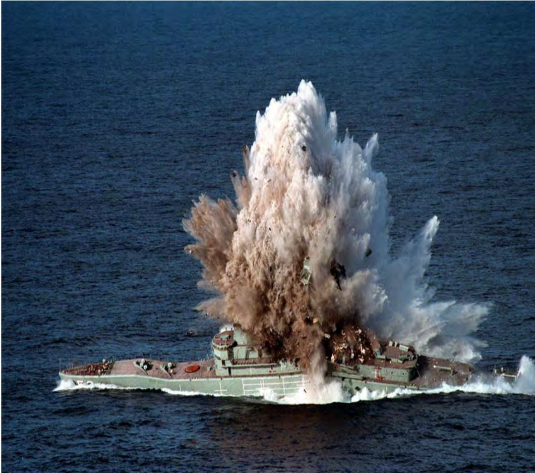
**Figure 5. The Keel Has Broken**
