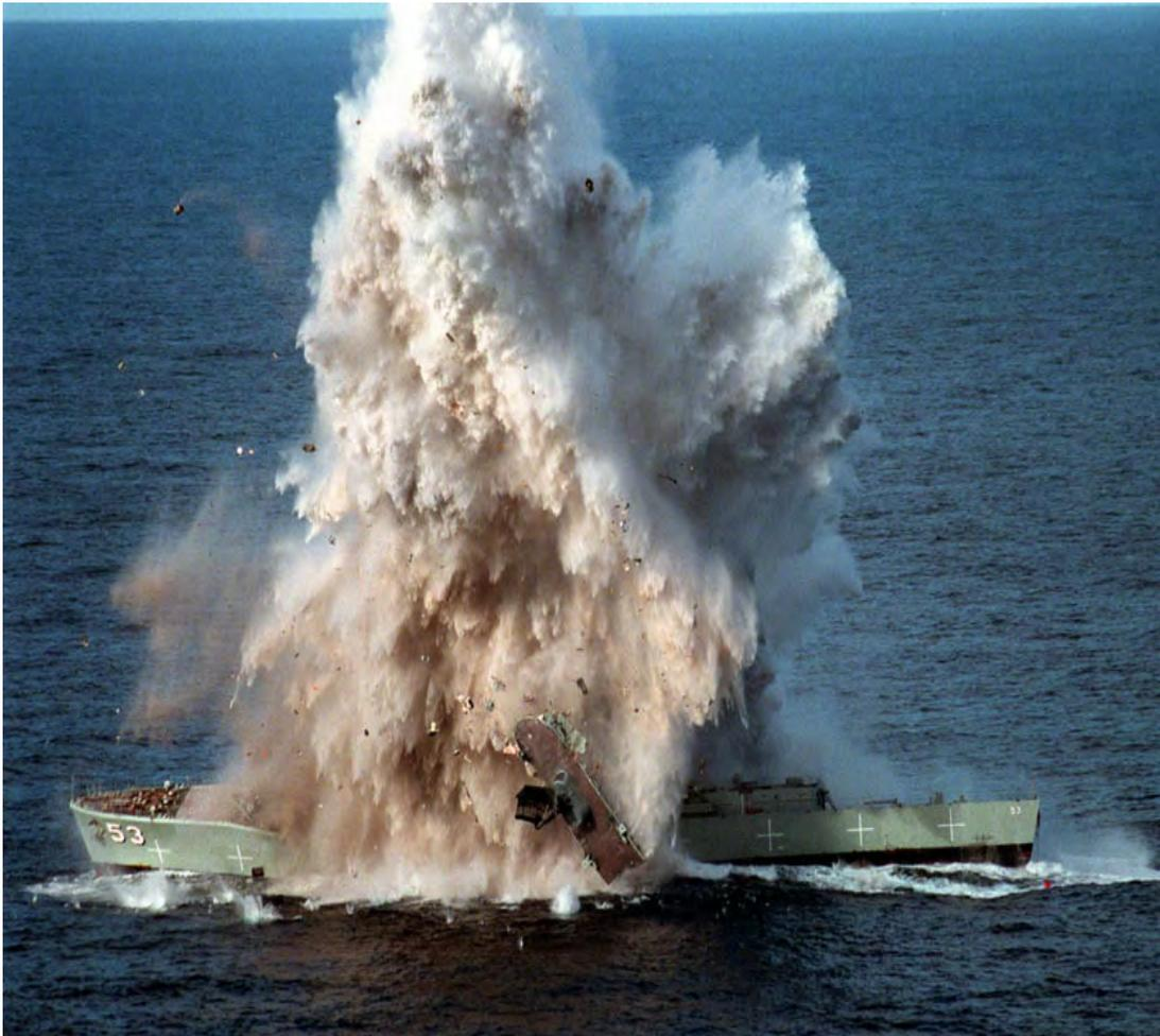
**Figure 6. Bow and Stern Sections Separate**
