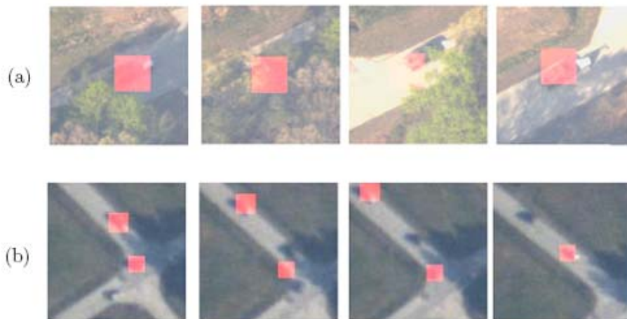
Figure 6: Instances of occlusion: (a) successful recovery from tree occlusion, (b) unsuccessful encounter with environmental shadows, with subsequent confusion of one vehicle for another
