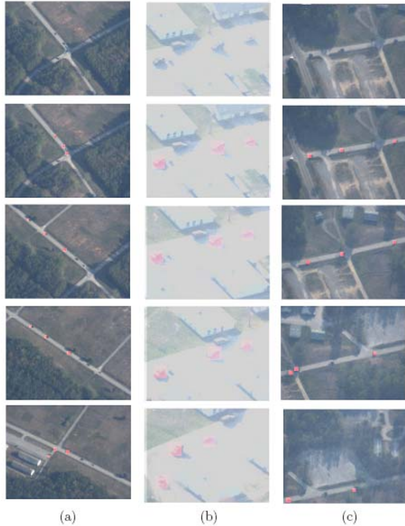
Figure 5: The tracker highlights vehicles on the image using a transparent red mask.
