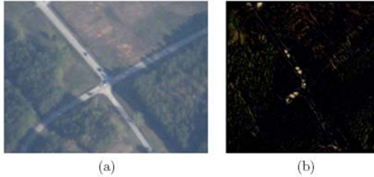
Figure 3: Intermediary output of detection: (a) visible frame, (b) corresponding vehicles highlighted as pairs of bright 'blobs'
