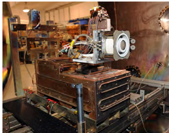
(b) The null-type inverted pendulum thrust stand used for performance measurements.
