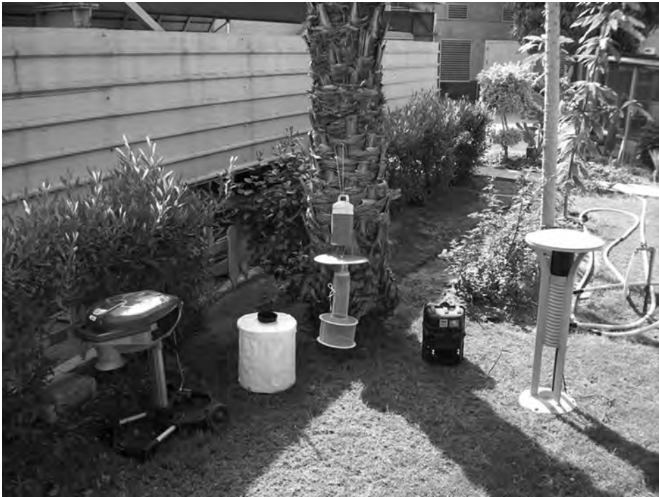
Fig. 1. Traps tested for sand fly capture (left to right): the MMP, the BGS, CDC light trap, the MCU, and the S360.
