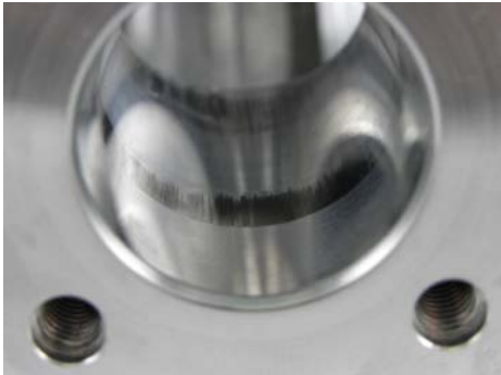
Figure 9 – Post-test SPK Pump Body Bore Polish
