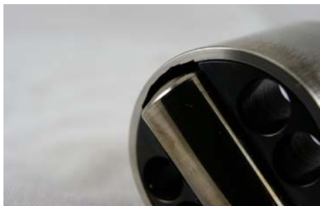
Figure 7 – Roller Wear into Follower, 50/50 JP-8/SPK
