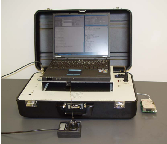
Figure 3. Portable Gateway Station (PGS), Host for NCC Software
