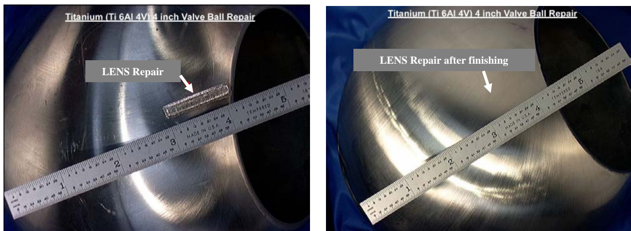
Figure 12. Submarine Cooling System Ti 6-4 Ball Valve repaired with LENS®.
