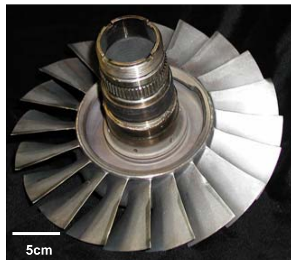
Figure 14. Blisk repair, post finishing, for T700 Engine.
