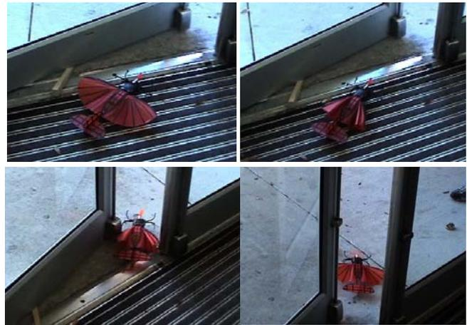
Fig. 6: When (a) MMALV is confronted with a narrow passage, it (b) retracts its wings, (c) negotiates the passage, and (d) redeploys its wings.
