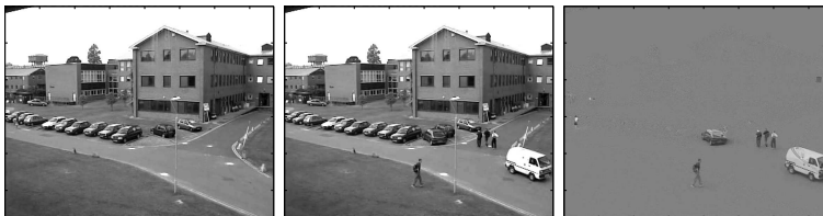
Fig. 1. (Left) Example background image. (center) Test image. (Right) Difference image. Note that the vehicle appearance also shows the curb in the background, which it occludes. The images are from the PETS 2001 database.
